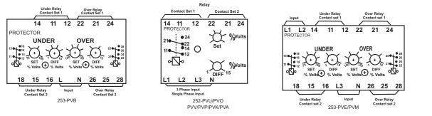
Note : The neutral connection is always used on 4 wire system
