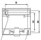
2 FIXING HOLE 'A' TO SUIT M4 / 2 FIXING HOLE 'B' TO SUIT M5
