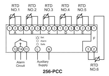
When used for less than 6 RTD inputs the unused terminals 1,2 & 3 must be linked together.
