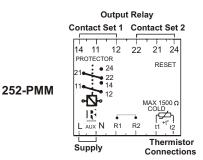
252-PMM can operate in either an automatic or a manual reset mode. For automatic the reset link R1-R2 is to be disconnected. For manual the reset link R1-R2 must be inserted.
