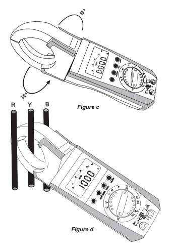
Normally, it is difficult to access the middle busbar for current measurement. With "Rotary mechanism for clamp jaws" it is easy to access middle bus bar, while keeping display and keys facing towards the user as shown in **figure d** on previous page.
