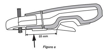
User's hand is at safer distance from bare bus bar/conductor.
