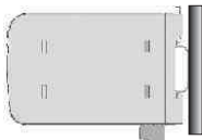
Fig. 3 Top-hat rail Mounting
