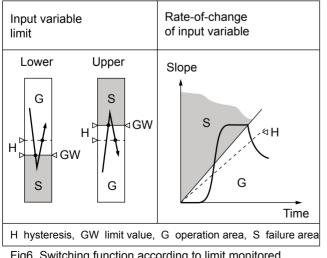
Fig6. Switching function according to limit monitored
