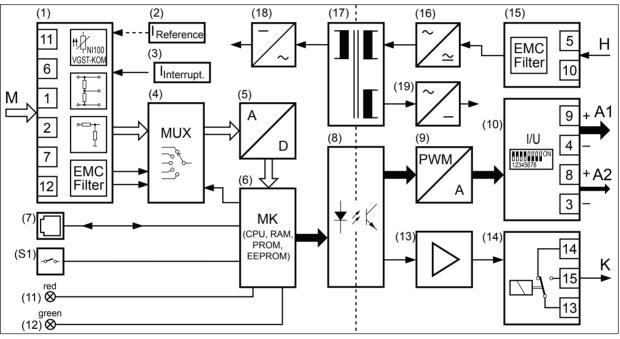
Fig. 3. Block diagram. I
