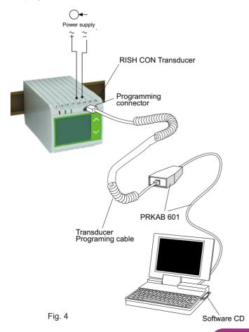
The Configuration software is supplied on a CD. The programming cable PRKAB601 adjusts the signal level and provides the electrical insulation between the PC and RISH CON Transducers.
