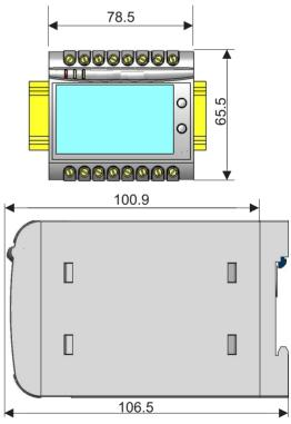
Fig 3. ( All dimensions are in mm.)
