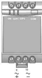
Fig. 6 Aux Terminal allocation
