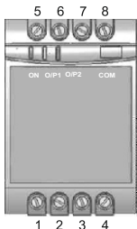
Fig. 5 Input & Output Terminal allocation
