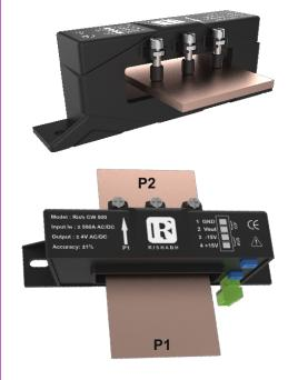
a) It is recommended to fix the primary busbar at the center of the aperture as the accuracy of the transducer is influenced by the position of the busbar.
