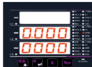
Screen 5 : Apparent Energy
