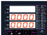
Screen 4 : Reactive Energy (Capacitive)
