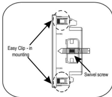
As the front of the enclosure conforms to IP 50, additional protection to the panel may be obtained by the use of an optional panel gasket. The terminals at the rear of the product should be protected from liquids.
