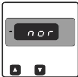
This screen is used to set the meter type. The user can scroll between the following options using the “ $\Delta$  up” key
