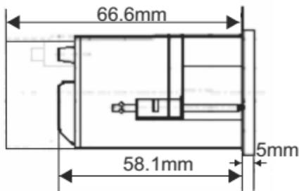
**For 48 x 96mm-**Mounting of Rish Eine+ DC DPM 48 x 96 is featured with easy "Clip- in" mounting. Push the meter in panel slot (size 48.5 x 96 mm), it will click fit into panel with the four integral retention clips on two sides of meter. The front of the enclosure conforms to IP54. Additional protection to the panel may be obtained by the use of an optional panel gasket. The terminals at the rear of the product should be protected from liquids.
