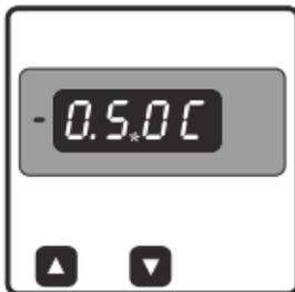
After entering the edit mode, by pressing the "  $\Delta$  " key user can turn the '-' symbol On or Off. If '-' symbol is On then PF Start value will be set as negative else it will be positive. 'L' (inductive) or 'C' (capacitive) are automatically displayed depending on the quadrant in which value is being set. Pressing the "  $\nabla$  " key will set the '-' symbol and digit editing will start.
