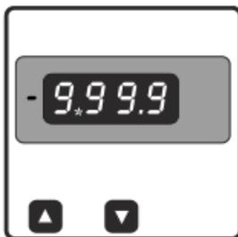
After entering the edit mode, by pressing the "△" key user can turn the '-' symbol On or Off. If '-' symbol is On then Display End value will be set as negative else it will be positive.
