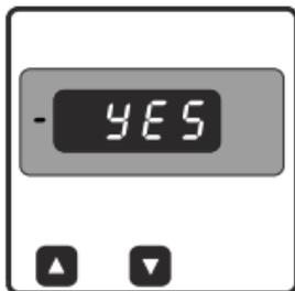
Initially, 'bEnt' message is displayed on screen. On pressing the "  $\Delta$  " key, the meter will enter the Bent function edit mode and user can scroll between yes and no. **YES:** Bent function is enabled
