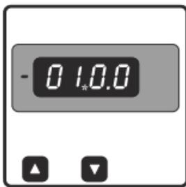
Initially, 'dSP.b' message is displayed on screen following which user can start editing Display Bent value by pressing the "△" key.
