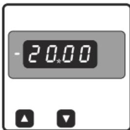
Initially, **"inP.S"** message is displayed on screen following which user can start editing Input Start value by pressing the " $\Delta$ " key.
