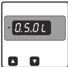
After entering the edit mode, by pressing the " $\Delta$ " key user can turn the '-' symbol On or Off. If '-' symbol is On then PF End value will be set as negative else it will be positive. 'L' (inductive) or 'C' (capacitive) are automatically displayed depending on the quadrant in which value is being set.
