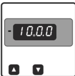
After entering the edit mode, by pressing the "  $\Delta$  " key user can turn the '-' symbol On or Off. If '-' symbol is On then Display Start value will be set as negative else it will be positive.
