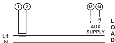
Connection For Ammeter DPM
