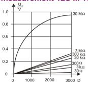
Voltage U<sub>x</sub> across the resistance R<sub>x</sub> to be measured as a function of measuring range and display.
